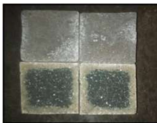
Figure: View of specimens showing Chloride Penetration
